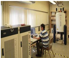
μMRI Bruker 7T/8.9cm (~ 10μm in 2D)
